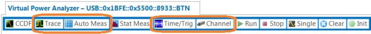
Figure 3.7 Use the Trace button on the Main Toolbar to display and setup a pulse measurement
